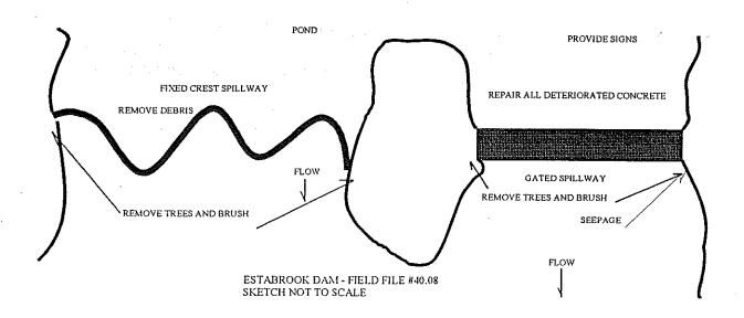
Due to the extent of the needed repairs, Milwaukee County will have to hire an engineer, registered in the State of Wisconsin, to design the repair of the dam. Plans must be submitted to this office prior to their implementation.
